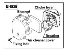
Dirty air cleaner element will cause starting difficulty, power loss, engine malfunctions, and shorten engine life. Keep the air cleaner element clean.
