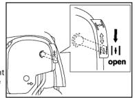
If engine fails to start after 5 or 6 pulls. Leave the choke lever on full choke. Lightly feather the throttle as you pull the rope.
