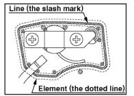
After cleaning, reassemble the air cleaner cover insert the tab at left, then insert the right tab and tighten fixing bolt
