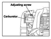
When the adjusting screw is turned right, engine rpm increases, and when it is turned left, rpm decreases. Never have auger rotation at idle.
